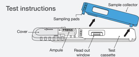
1 Slide the cover in the direction of the arrow until the word PRESS is entirely visible.
